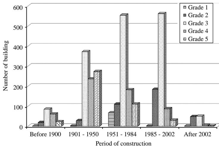
**Figure 3.** Diagram depicting distribution of the buildings falling under different damage grade classes with respect to their period of construction
