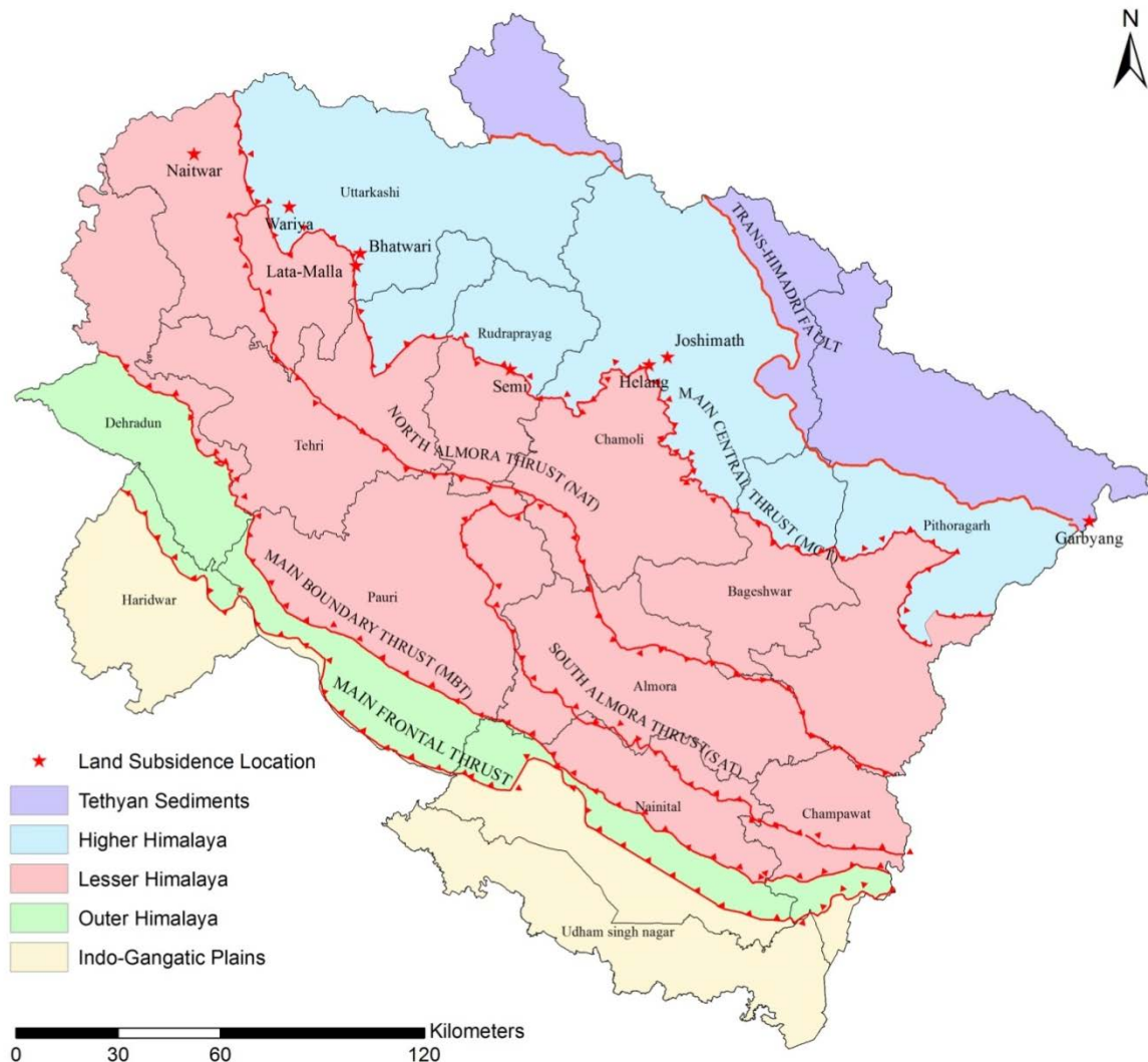
Fig. 6. Land subsidence along with chronic landslide zones located close vicinity to major structural dislocation (MCT) in Uttarakhand
