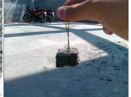
Fig. 46: An individual spacer.
