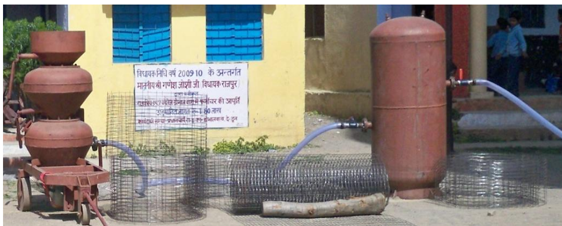
Fig. 49: Dry mix holder (left) and compression chamber (right).
