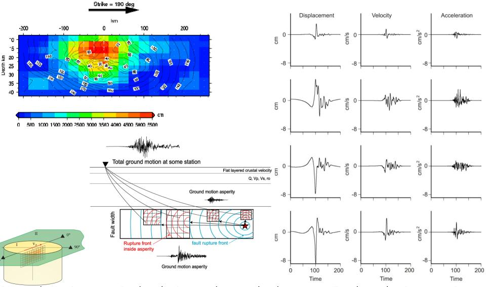
Ground Motion at a Bedrock site underneath due to an Earthquake Rupture is calculated by vectorial addition of the Finite Rupture response contributed by each cell as the rupture front runs along the fault.
