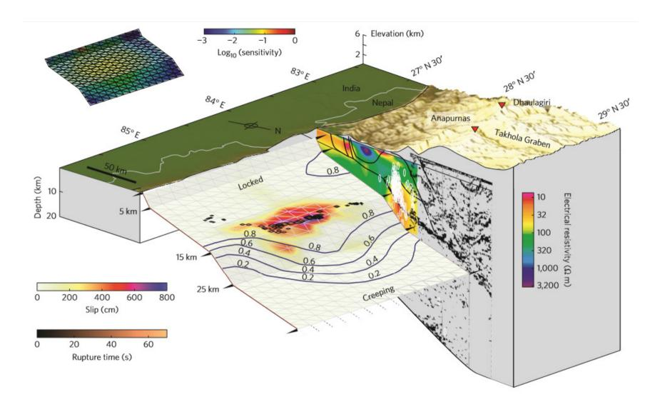
The 3D Decollement shows high frequency earthquake sources running along the ramp-flat hinge line rupturing the MHT at  $\sim$  15 km depth. The right wall shows the seismic reflection profile delineating faults & conducting (fluidized) zones Elliot et al., 2017
